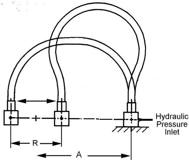
Figure 8B.1: Flex-impulse Testing Fixture
