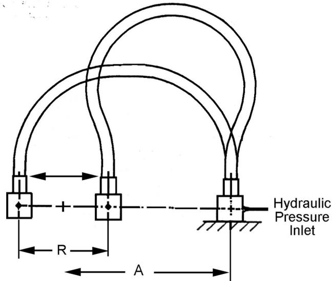
**Figure 8B.1:** Flex-impulse Testing Fixture
