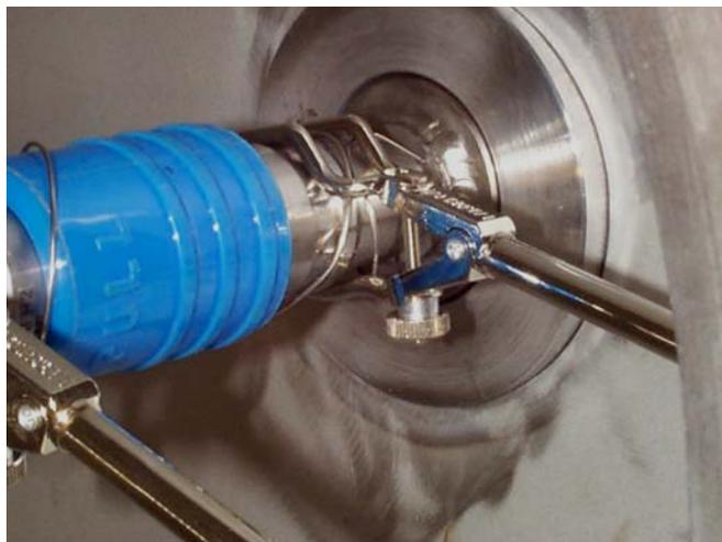
Figure 4. Fitting of thermocouples to the connector.
